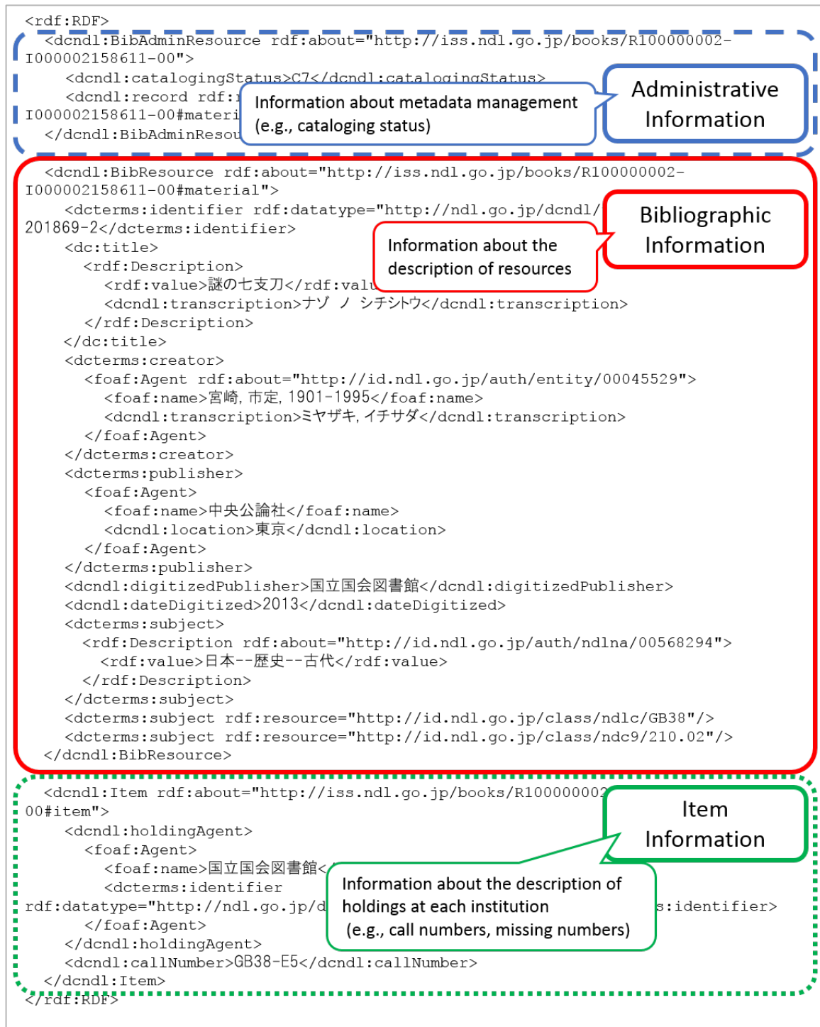
FIG. 1. Basic structure of the DC-NDL
